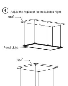
If the installation surface is too narrow, we suggest making the two fixing parts near to each other, please refer to drawing below.
